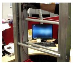
6. Raise platform above desired height by lifting from side of platform and slowly lower. Platform will lock into position resting on runglocks.
