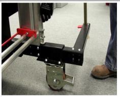
4. Lower stabiliser leg upright by lifting spring loaded catch and letting upright drop. Make sure upright is in firm contact with the ground and release catch.
